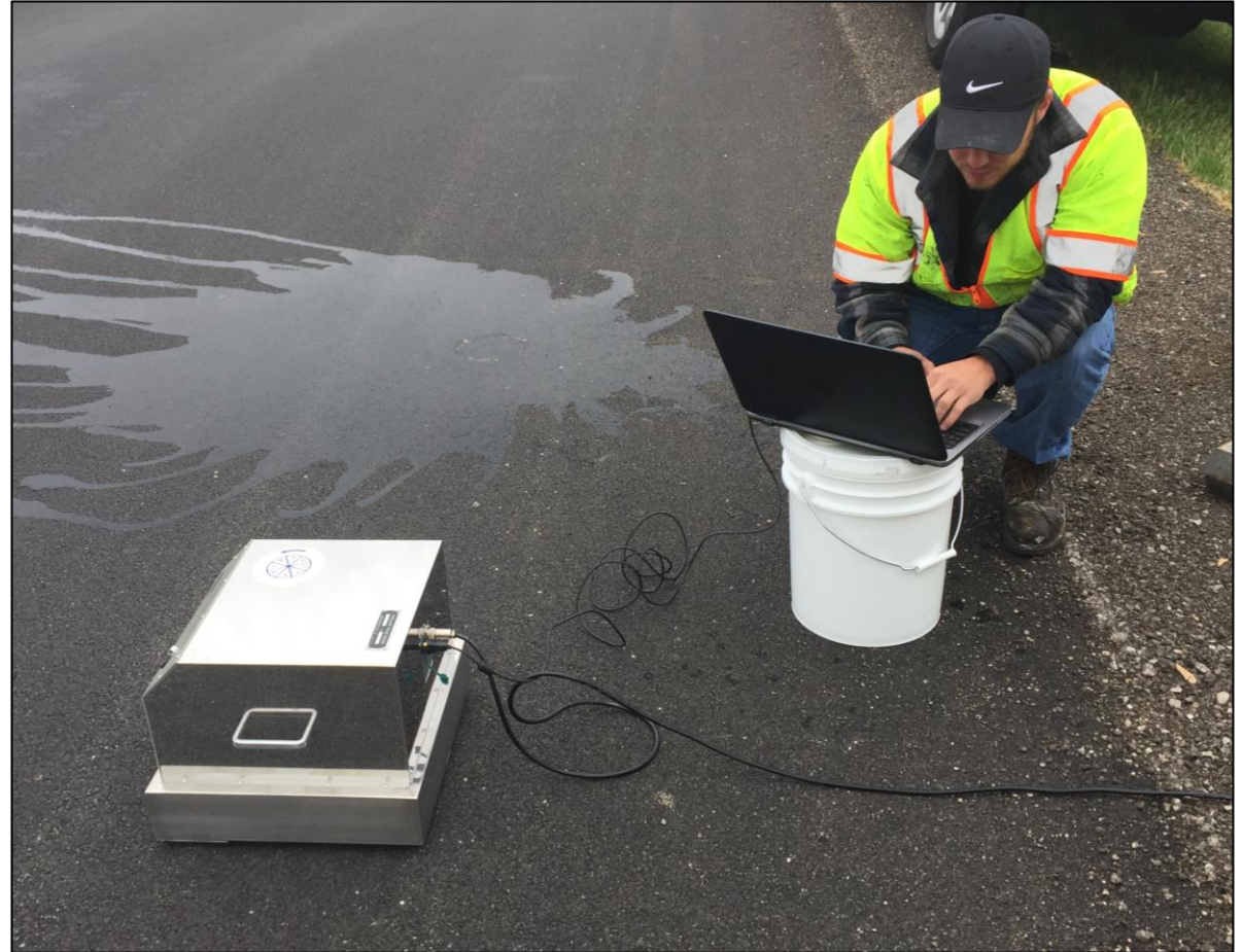
Circular Track Meter ASTM E-2157
