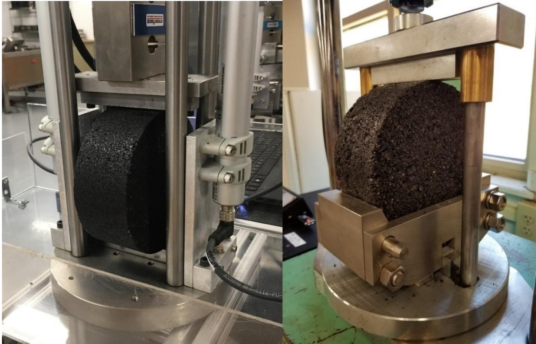
Figure 4. IDEAL-CT (ASTM D8225-19, left) and IDEAL-RT (ASTM D8360-22, right)
