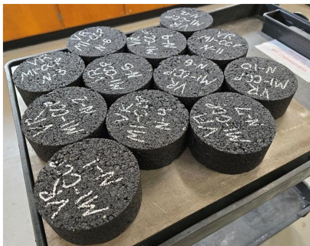
Figure 2. Compacted Asphalt Specimens – Dwell Time
